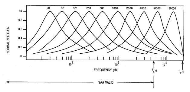
Figure 11. 10-Band Bandpass IIR Filter Response
