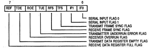
Figure 4. Read-Only SSI Status Register (X:\$FFEE)
