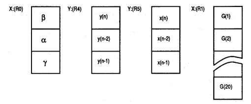
Figure 10. IIR Filter Data Structures
