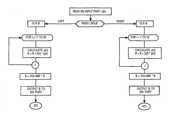
Figure 14(b). Algorithm Flowchart for CDP Interface and IIR Filter Processing (Interrupt Routine)
