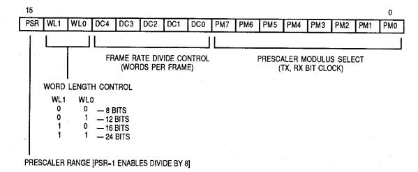
Figure 5. SSI Control Register A (X:\$FFEC)
