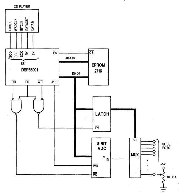
Figure 7. Block Diagram of DPS56001 Graphic Equalizer
