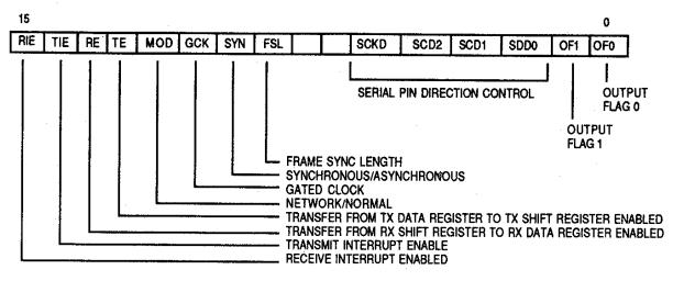
Figure 6. SSI Control Register B (X:\$FFED)
