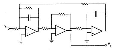
Figure 1(b). Op-Amp Active Bandpass Filter
